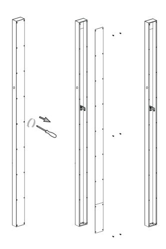
Use the screwdriver to unscrew the screws at the back of shower tower body and take out the back cover 1 and back cover 2.
