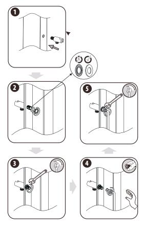
Fit the seal into the nut end of the shower hose and connect the nut to the outlet on the hand shower holder and tighten, if using a spanner, place a cloth around the nut to prevent damage.
